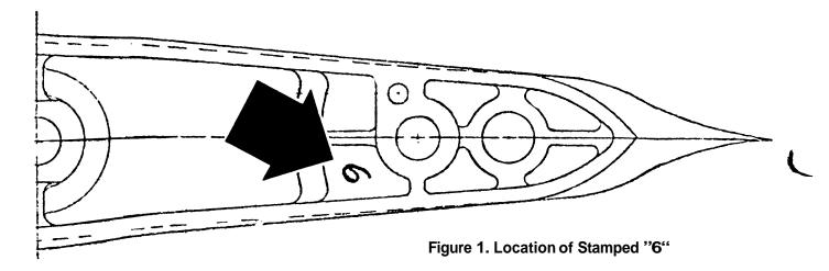
The "6" marking will identify a Merc 650 (3-Cyl.) gear housing from a Merc 500 or a Merc 402, which appear identical externally. To identify gear housing assemblies, which were manufactured previous to March 16,1972, turn the drive shaft one complete turn. If the propeller shaft turns only one-half (%) turn, the gear housing is a Merc 500-402 (2:1 gear ratio). The Merc 650 has a 1.65:1 gear ratio.
