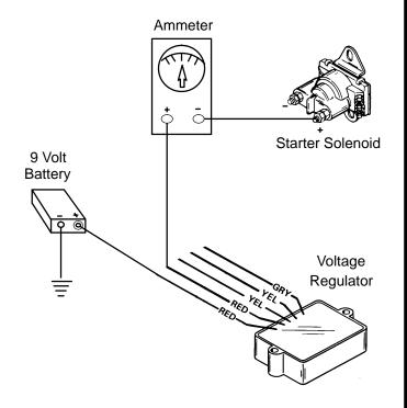
To Test Regulator: Ammeter and 9 volt transistor battery are required.
