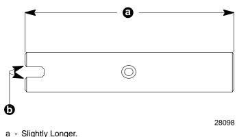
b - Chamfer Removed.
