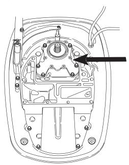
The replacement oil pump, Mercury part number 858579T3, has a painted green dot on the forward end and a date code ink stamped on the bottom. Please refer to the INSPECTION/ TEST section following for appropriate markings and date code. Oil pumps in dealer inventory identified by Mercury part numbers 858579, 858579T1, and 858579T2 should be returned to Mercury for credit.
