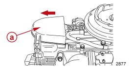
2. Remove camshaft driven gear bolt and washer.
