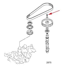
3. Install new washer and torque the driven gear bolt to specification.
