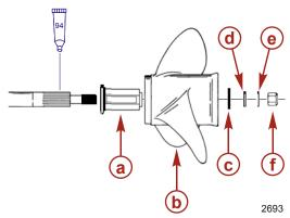
Propeller hardware 19 spline, 32 mm (1-1/4") propeller shaft
