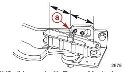
Shift slide used with Torque Master lower unit
