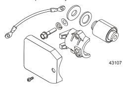
When servicing the lower mount cover or clamp with the single screw design, please order P/N 879150A90 cover kit. The kit will include the cover, the mount clamp, and three screws to secure the cover to the clamp.
