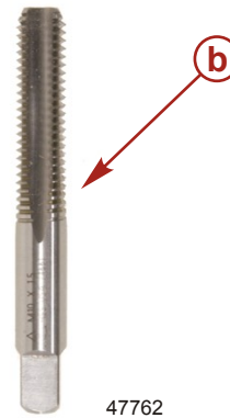
a - Upper knock sensor mounting boss tapping operation b - 10 x 1.5 mm bottoming tap (obtain locally)
