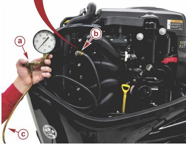
5. Turn the ignition key off and then on. The fuel pumps will run for approximately three to five seconds. Continue this ignition key cycle until the purged fuel is relatively clear of air bubbles.
