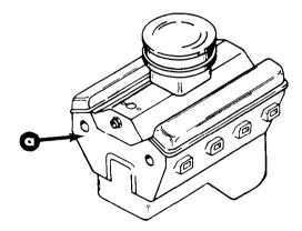
V6 (Front, Starboard Side, Near Cylinder Head Mating Surface) - T02280KP/KR - T05290KPIKR February 28, 1990 to May 29, 1990 build date
