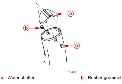
The water shutters should be inspected every 300 hours or 3 years as part of routine maintenance. Replace the water shutters as required.
