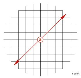
1.15 mm (0.045 in) galvanized steel, 12.7 mm (1/2 in) mesh screen
