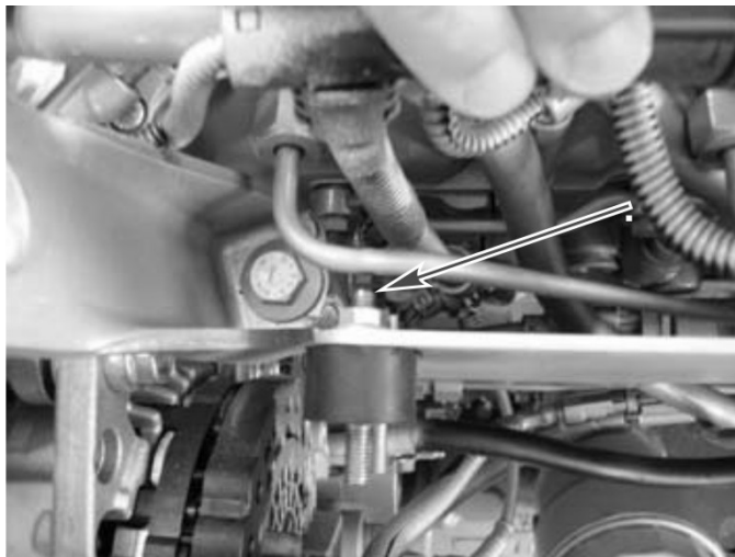
Vibration damper with short stud toward engine
