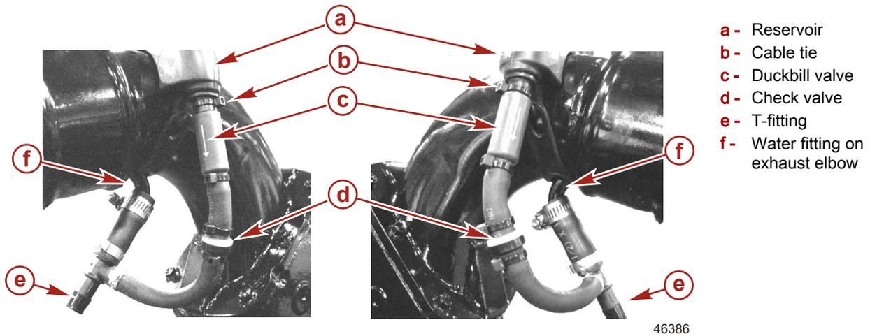
8. Inspect the grommet-to-reservoir area to assure there is no side-load pulling on the grommet. The grommet should be relaxed and fully seated against the reservoir. The hose should not be bent or kinked. Position the T-fitting portion of the assembly as necessary to ensure proper assembly.
