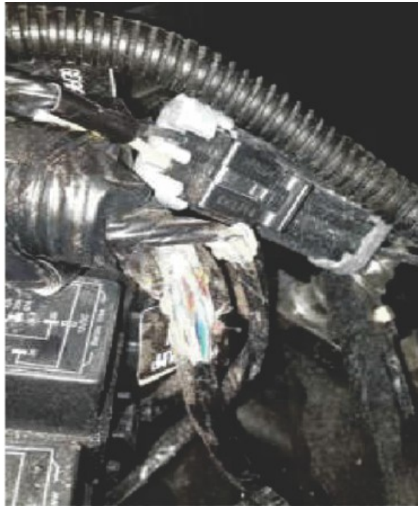
Example of damaged insulation and bare wire
