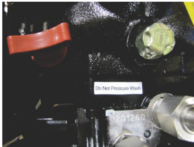
Transmission vent cap location
