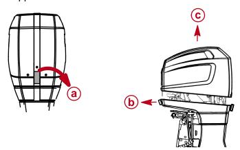
a - Rotate rear latching handle clockwise.
