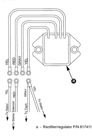
To correct this condition the tachometer lead must be connected to the Yellow rectifier/regulator lead that does not have continuity to the Gray rectifier/regulator lead. Test as follows to determine which Yellow lead to use:
