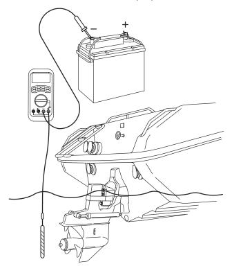
5. Record hull potential readings at this time.
