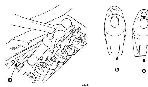
a - Push Rod Hole: Slot=Keeps Push Rod Aligned.
