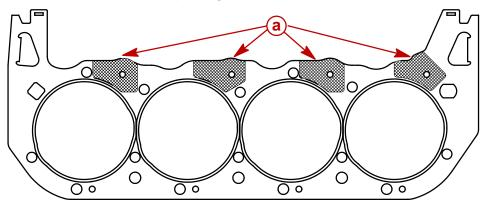
a- Sealing Material Around Upper Water Passage Holes
